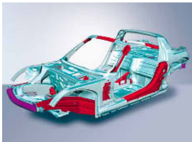
smart roadster: TRIDION cell body with structural reinforcements (red)
