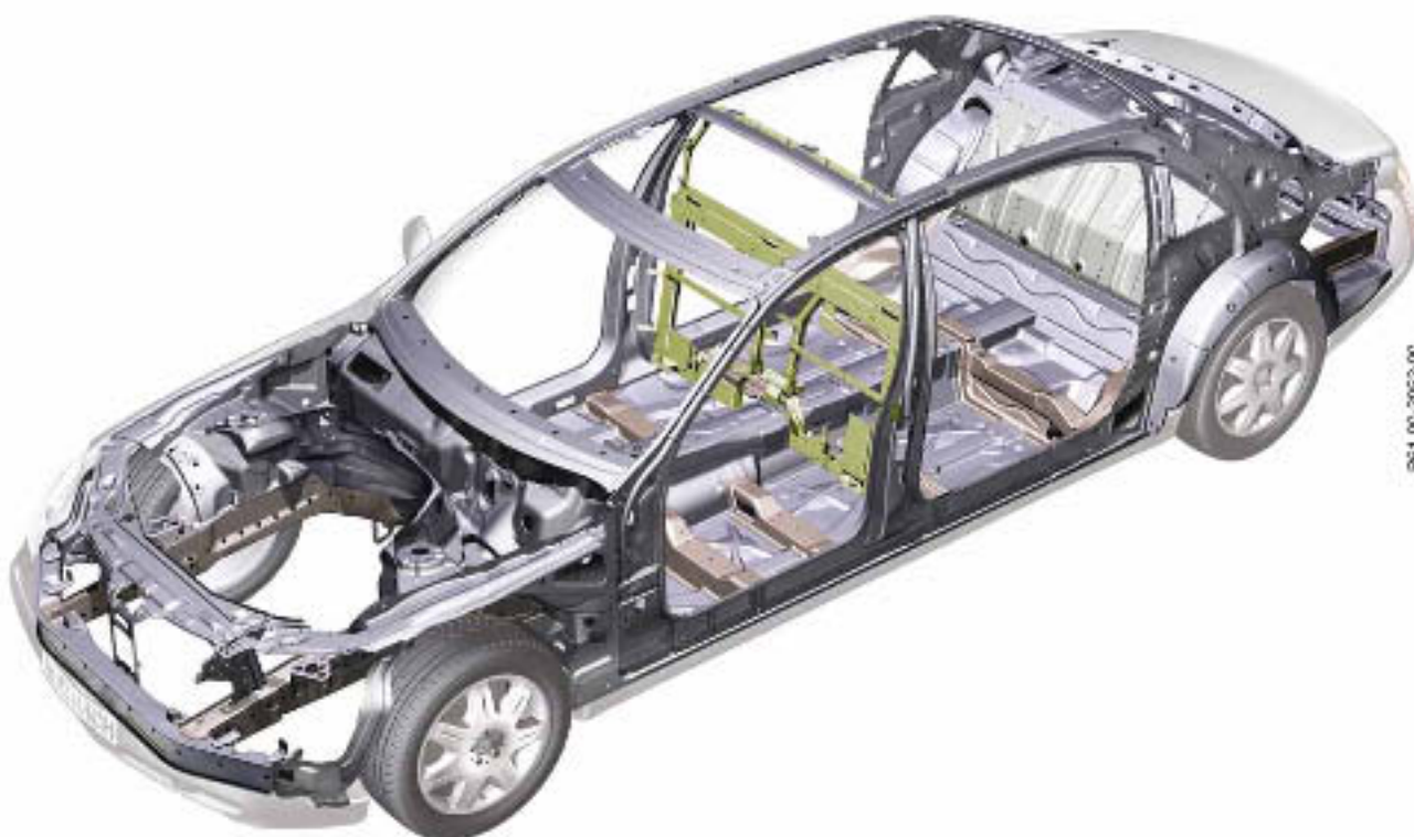
Bodyshell of Maybach 62 with partition wall (model 240)
