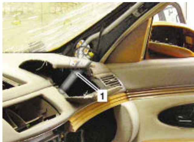
1 Right front windowbag gas generator
