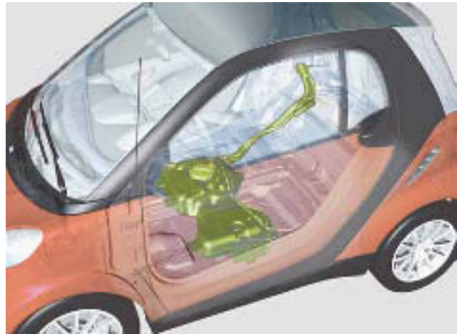
Fuel tank on smart fortwo (model 451)
