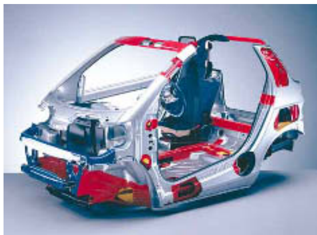
smart fortwo cabrio: TRIDION cell body with structural reinforcements (red)
