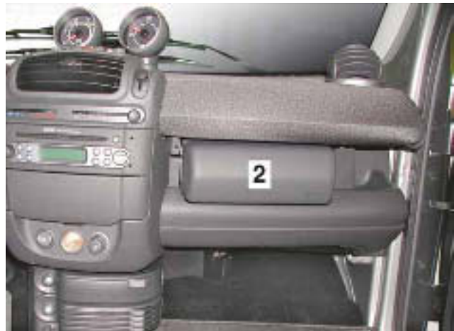
2 Front passenger airbag on smart fortwo (model 450)
