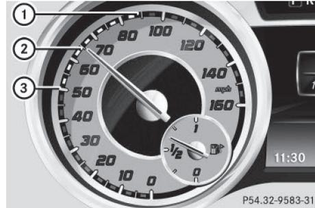
Example: DISTRONIC PLUS displays in the speedometer
