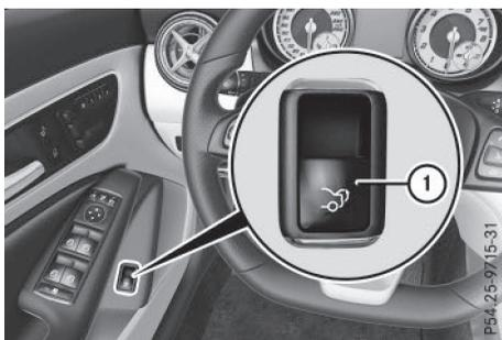
You can open the trunk lid from the driver's seat when the vehicle is stationary and unlocked.
