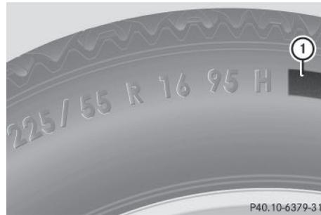
In addition to the load-bearing index, load index **①** may be imprinted after the letters that identify speed rating on the sidewall of the tire. Speed rating (▷ page 268).
